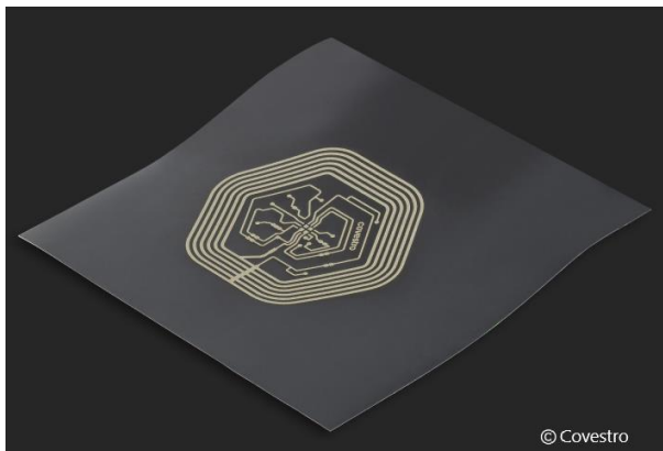
Printed electronics on Platilon TPU Film © Covestro
